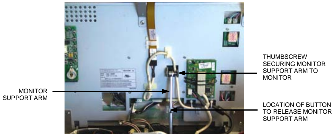
FIGURE 2 - SUPPORT ARM CONNECTION TO MONITOR
