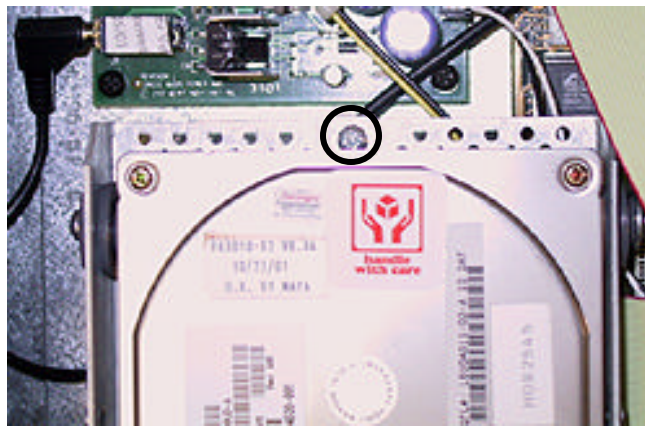
FIGURE 1 - HARD DRIVE REMOVAL - LOCATION OF SCREW SECURING HARD DRIVE MOUNTING PLATE TO CPU SHELF
