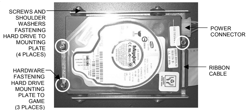
FIGURE 12 - HARD DRIVE IN MAXX TO FORCE CONVERTED GAMES
