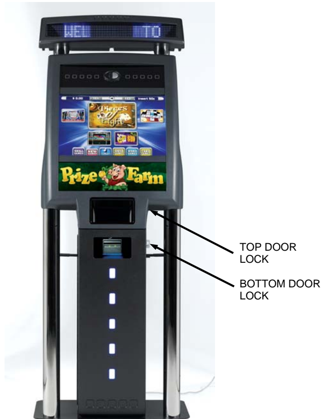
FIGURE 1 – PRIZE FARM CABINET DETAILING LOCK LOCATION
