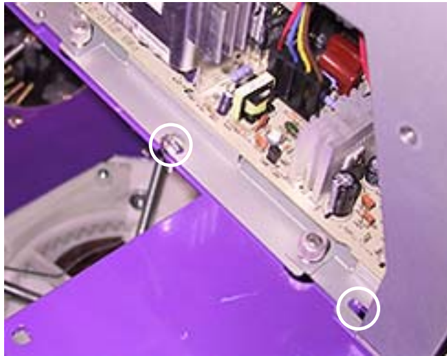
FIGURE 7 - POSSIBLE HARDWARE LOCATION FOR MOUNTING MONITOR
