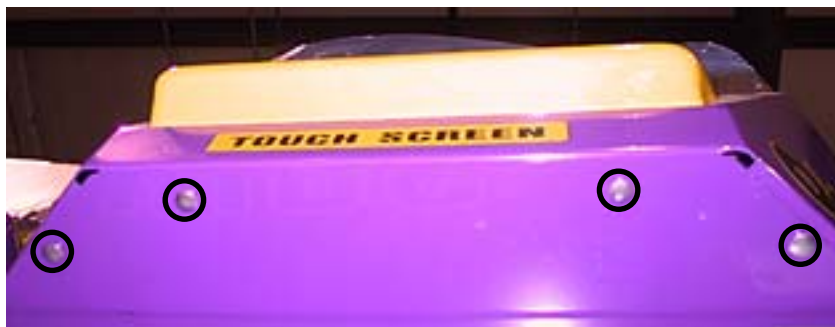
FIGURE 5 - FRONT OF SHROUD FASTENED WITH BOLTS
