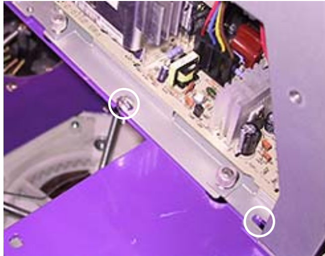
FIGURE 6 - POSSIBLE HARDWARE LOCATION FOR MOUNTING MONITOR
