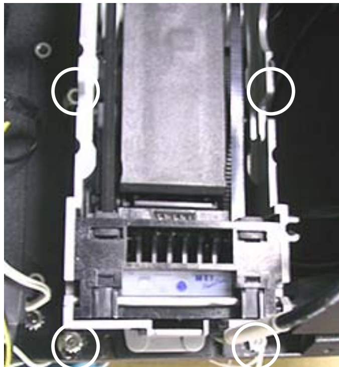
FIGURE 4 - SCREWS SECURING BILL ACCEPTOR TO MOUNTING PLATE
