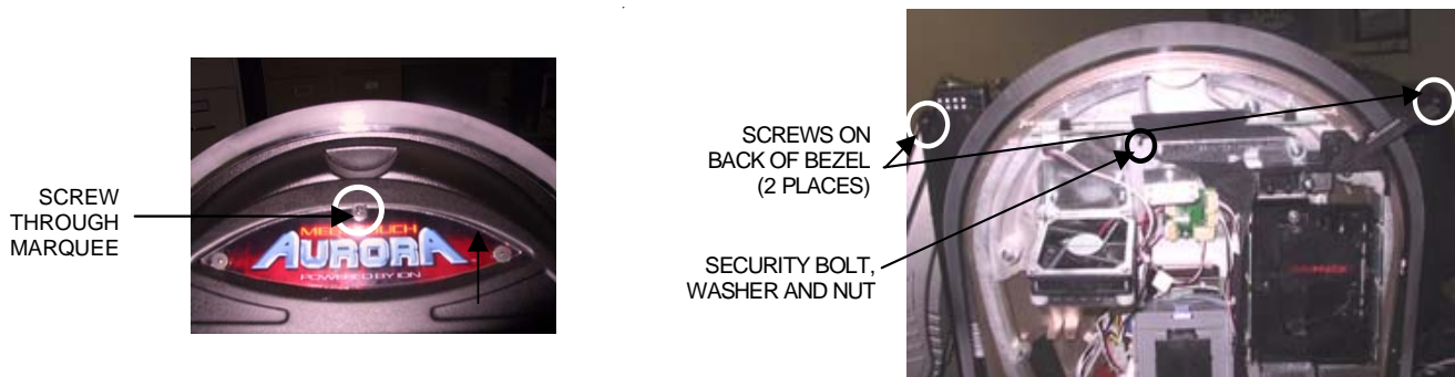
FIGURE 3 - SCREWS ON FRONT AND BACK OF BEZEL
