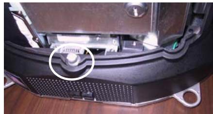
FIGURE 2 - SCREW IN CENTER OF BOTTOM COVER
