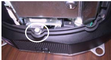
FIGURE 2 - SCREW IN CENTER OF BOTTOM COVER
