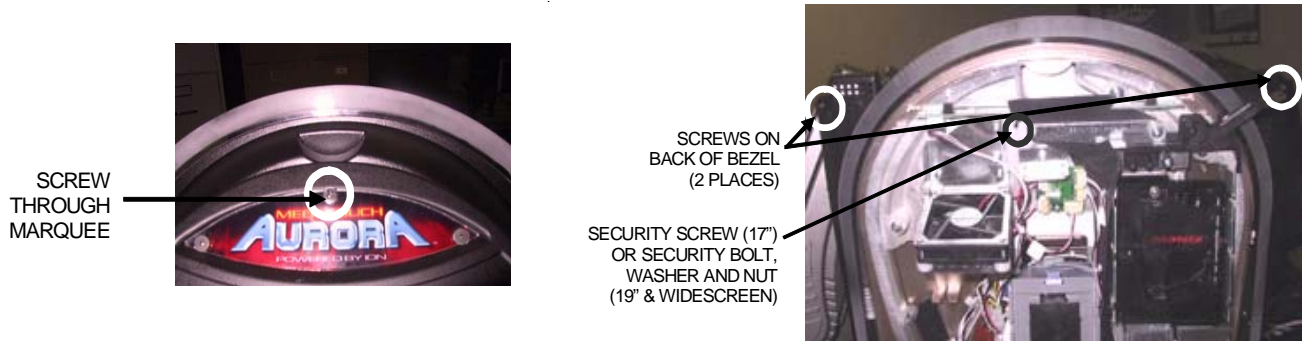
FIGURE 4 - SCREWS ON FRONT AND BACK OF BEZEL
