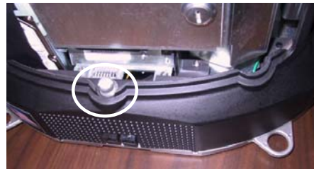
FIGURE 1 - ROTARY DRAW LATCH INSIDE TOP COVER FIGURE 2 - SCREW IN CENTER OF BOTTOM COVER
