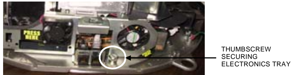
FIGURE 10 - REAR VIEW OF ELECTRONICS TRAY
