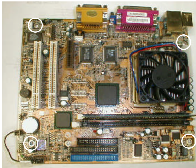
FIGURE 1 – MOTHERBOARD REMOVAL – LOCATION OF SCREWS SECURING MOTHERBOARD TO MOUNTING FRAME
