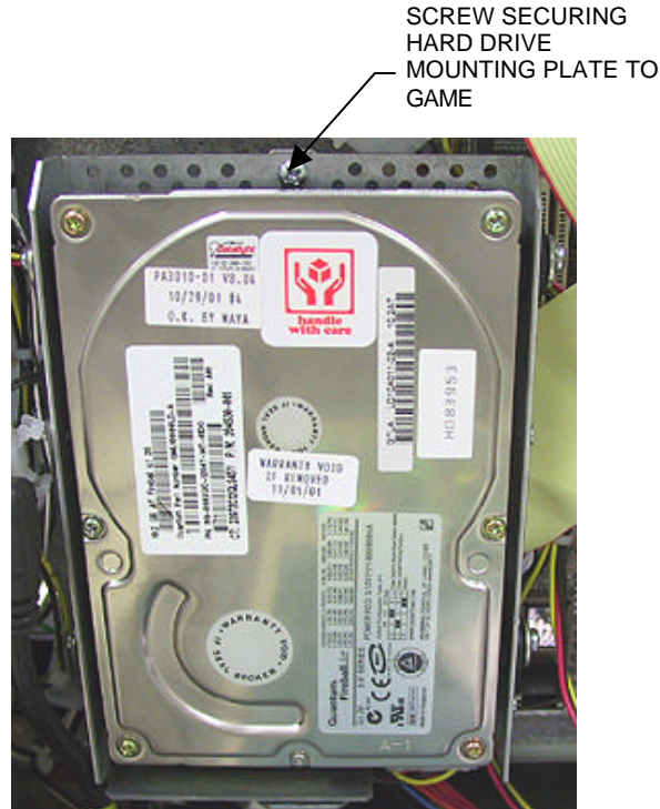
FIGURE 1 – HARD DRIVE REMOVAL
