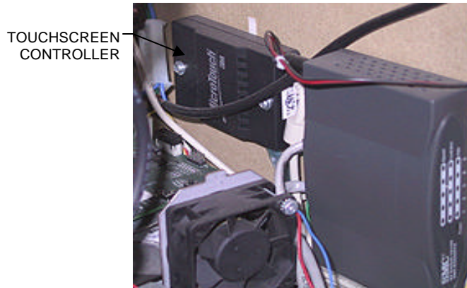
FIGURE 1 - MEGATOUCH COMBO JUKEBOX - INSIDE REAR OF CABINET
