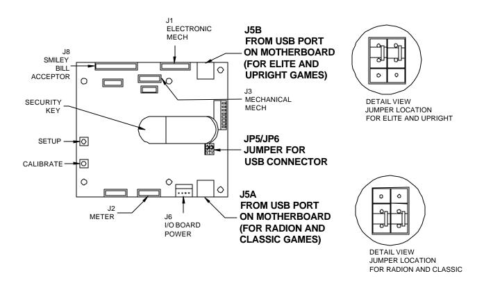
FIGURE 1 - MEGATOUCH FORCE I/O BOARD DRAWING
